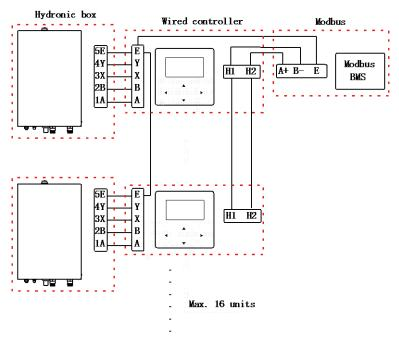
Note: Wired controller is integrated in the hydronic box.
