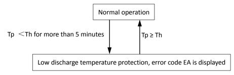
When the discharge temperature is lower than suction temperature for more than 5 minutes, the system displays EA protection and the unit stops running. When the discharge temperature is higher than suction temperature, the compressor enters re-start control.
