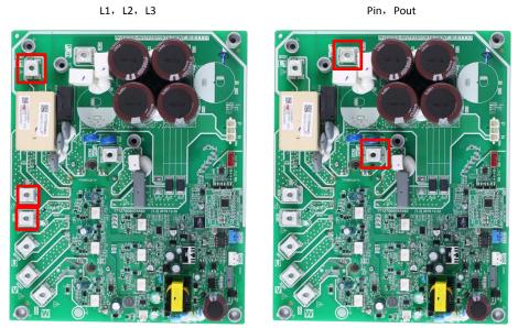
2. The normal resistances of the inverter compressor are  $0.7-1.5\Omega$  among U V W and infinite between each of U V W and ground. If any of the resistances differ from these specifications, the compressor has malfunctioned.
