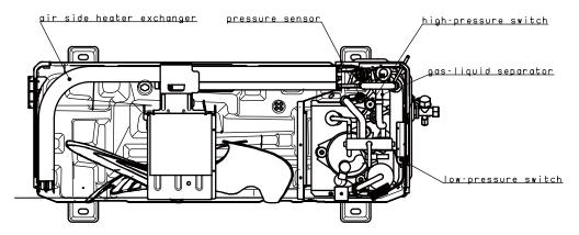
Figure 2-1.2: MHA-V4(6)W/D2N8-B front view
