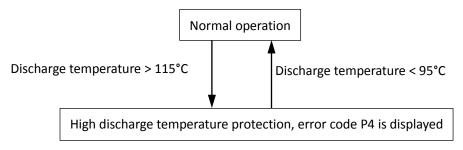
When the discharge temperature rises above 115°C the system displays P4 protection and the unit stops running. When the discharge temperature drops below 95°C, the compressor enters re-start control.
