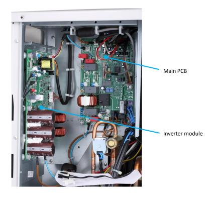
Figure 4-1.3: MHA-V12(14,16)W/D2N8-B electric control box
