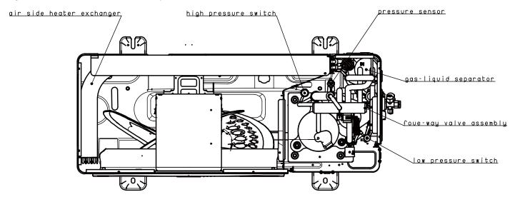
Figure 2-1.6: MHA-V12(14,16)W/D2N8-B front view
