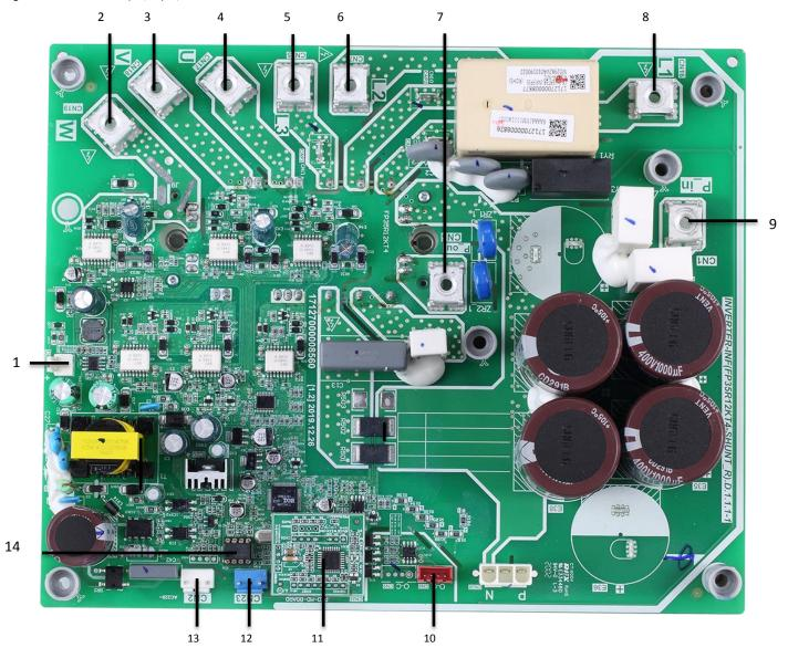
Table 4-2.7: MHA-V12(14,16)W/D2RN8-B outdoor unit inverter module
