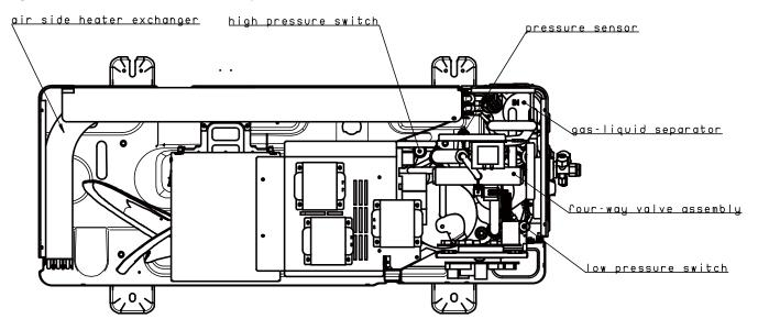
Figure 2-1.8: MHA-V12(14,16)W/D2RN8-B front view
