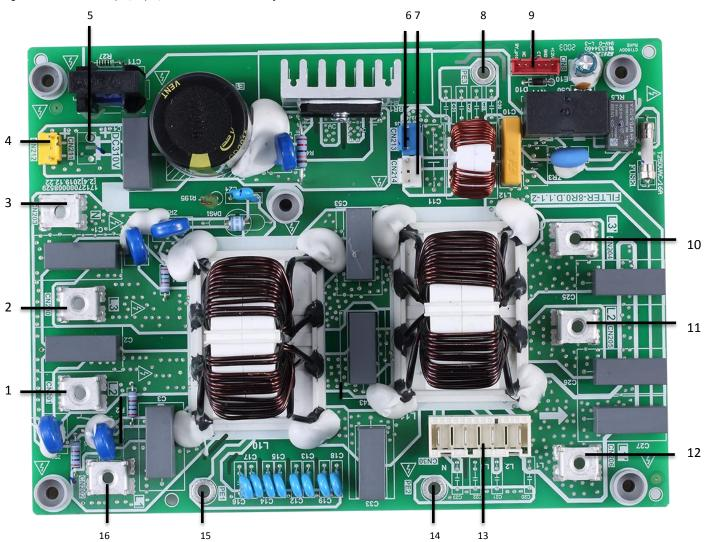
Table 4-2.8: MHA-V12(14,16)W/D2RN8-B outdoor unit filter board
