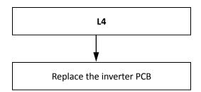
Condition 2: L4 error appears after the compressor has been running for a period of time and the compressor speed is over 60rps
