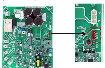
Figure 4-4.8: Connection port for inverter module
