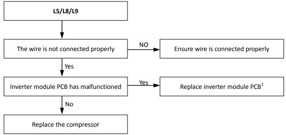
1. When replacing an inverter module, a layer of thermally conductive silica gel should be painted on IPM module (on the reverse side of the inverter module PCB). Refer to Figure 4-4.2.
