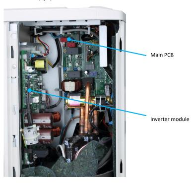
Figure 4-1.2: MHA-V8(10)W/D2N8-B electric control box
