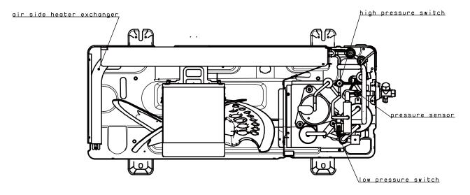
Figure 2-1.4: MHA-V8(10)W/D2N8-B front view
