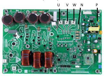
Situation 1: L1 or L2 error appears immediately after the outdoor unit is powered-on
