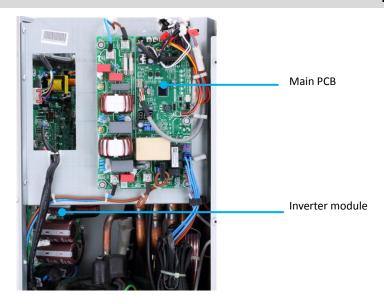
Figure 4-1.4: MHA-V12(14,16)W/D2RN8-B electric control box
