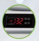
The digital controller features visual and acoustic alarms, high/low-temperature alarms, open-door alarms and a data logger.
